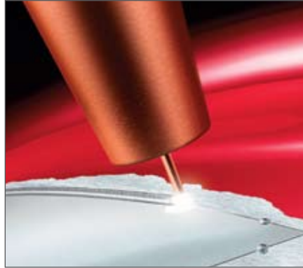
Thin sheet metal autobody work
